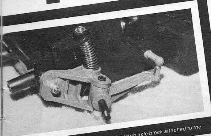
Above: the completed suspension assemblies fixed to the injection moulded chassis.
