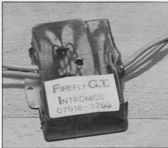
Left: the Intronics 'Firefly GT' speed controller, a must for the weight conscious racer. The photograph shows the unit oversize.
