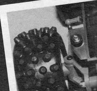
Right: steering servo-saver arrangement with servo in place.
